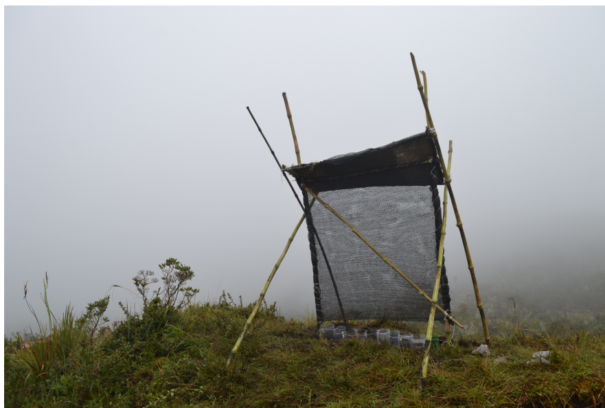
Figure 22: Horizontal precipitation station built to get a better understanding of the contribution of water from horizontal precipitation.
