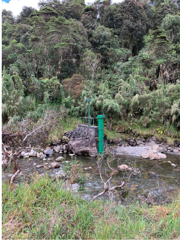
Figure 3: The limnigraph in green is continuously measuring the water level.
