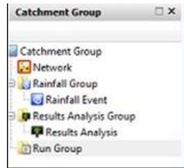
Figure 10; A screen shot from Infoworks of the workgroup structure when building a model with a network in the Catchment group, a rainfall event added in the Rainfall group and a Run group which is needed for making simulations.
