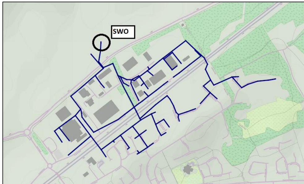
Figure 17; Map of the stormwater system with the outfall (SWO) marked (Map by OpenStreetMap 2014)
